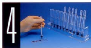
5 The sediment and stain are then mixed by gentle repeated squeezing of the KOVA Petter bulb. The petter is used to transfer one drop to the appropriately numbered chamber on either a four-well or ten-well KOVA Slide. Each chamber of all KOVA Slides contains a standard volume of 6.6 µL. Capillary action will draw this precise amount of urine into the slide chamber.
