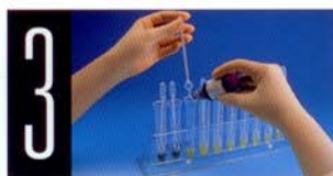
4 The KOVA Petter is withdrawn and one drop of KOVA Stain (Sternheimer-Malbin) is added to aid in the visualization of cells and casts (see KOVA Stain package insert for the staining characteristics of each sediment element).
