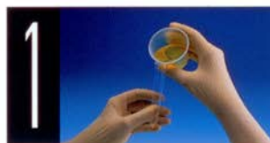
1 After sample collection and transportation to the laboratory, 12 mL of each of the specimen or the controls are poured into separate graduated KOVA Tubes. When the specific gravity and dipstick chemistries have been determined, the capped tubes are centrifuged at 1500 RPM (6" rotor = 400 rcf) for five minutes.
