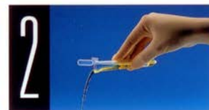
2 Tubes are then removed from the centrifuge and a lock tip KOVA Petter is firmly inserted into each tube trapping 1.0 mL of sediment; the supernatant is then decanted as shown.
